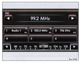
**Fig. 7** RADIO main menu with dial for the selected frequency band.
